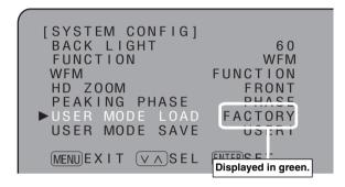
When the file whose data is to be loaded is selected from the FACTORY or USER1 to USER5 files and the FUNCTION/ENTER button is then pressed, the screen shown below appears.
